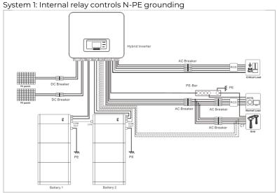
Figure 5-1 System Electrical Topology (General)
