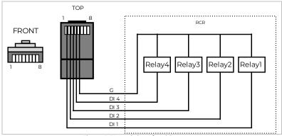
Figure 5-39 Logic interface(a)
