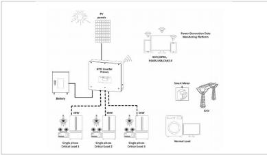
Figure 3-11 Unbalanced load (EPS mode)
