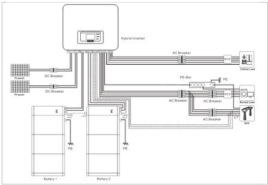
Figure 4-9 System with BTS 5K / RBS5000 battery
