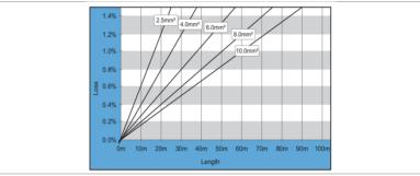
Figure 5-15 The relationship between the leakage power and cable length
