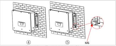
Figure 4-7 Installing HYD 5...20KTL-3PH(b)
