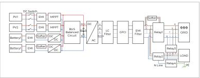
Figure 3-4 Electrical schematic diagram
