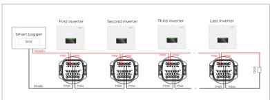
Figure 5-23 RS485 communication connection
