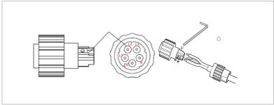
Figure 5-18 AC connection (c)
