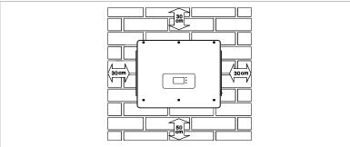
Figure 4-3 Minimum distances for individual inverter
