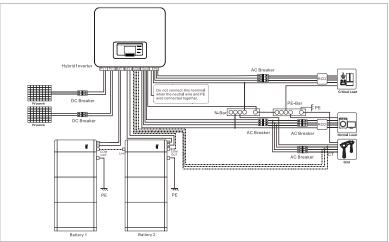
Figure 4-10 System with BTS 5K / RBS5000 battery in Australian N-Grid with N-EPS connected
