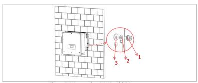
Figure 5-8 Connecting PGND cable(c)
