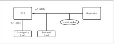
Figure 7-4 Schematic diagram of Genset Mode
