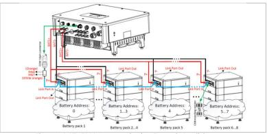
Figure 4-8 GTX 3000-H connecting in 4 Towers in Parallel
