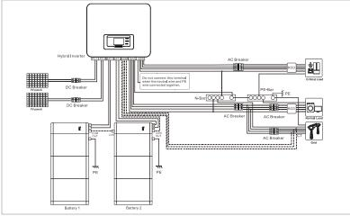
Figure 5-2 System Electrical Topology
